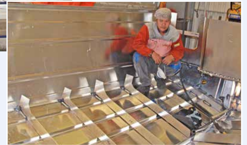
Left and below: Aluminium 'gibs' give strength and shape to the hull. A special TIG welding process ensures quality welding.
