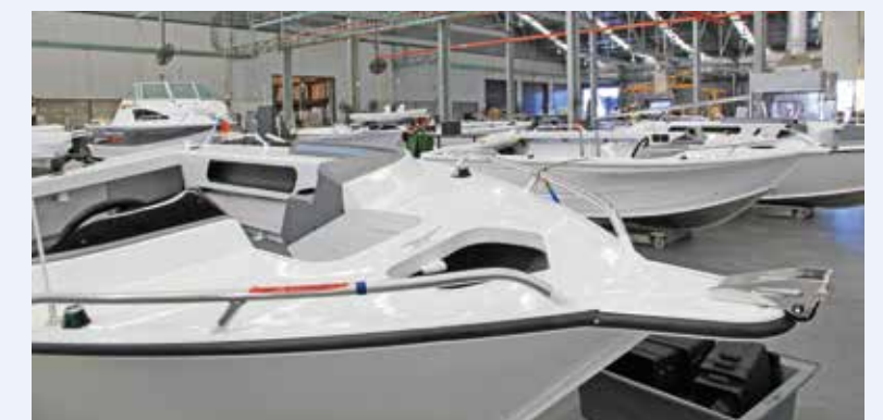
The larger plate models typically take around seven days to complete. Over 60 hours of welding goes into each boat.
